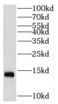
K-562 cells were subjected to SDS PAGE followed by western blot with FNab05880(NUTF2 antibody) at dilution of 1:500
