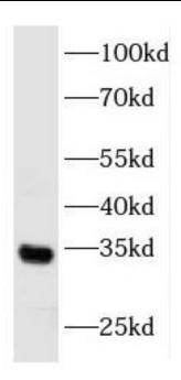
MCF-7 cells were subjected to SDS PAGE followed by western blot with FNab03092( FGF17 Antibody) at dilution of 1:600
