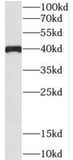
COLO 320 cells were subjected to SDS PAGE followed by western blot with FNab01121(C5orf4 Antibody) at dilution of 1:300
